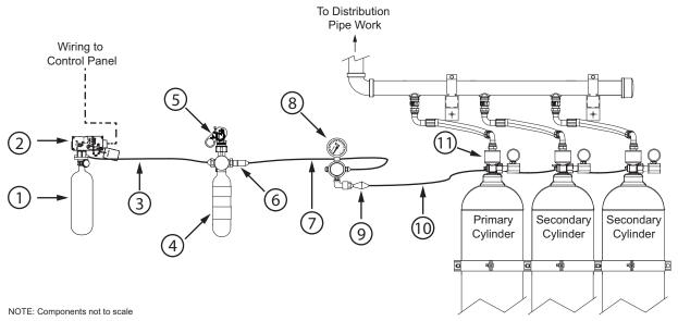
Figure 3. System with Discharge Delay
