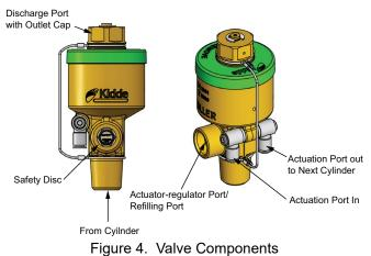
The Natura IGS valve assembly has a 3/4 in. (20mm) discharge port with BSP male threads.
