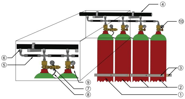
Figure 1. Single Area Cylinder Bank Arrangement
