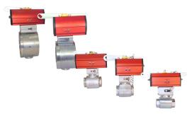
Figure 12. Selector Valve Selector valves are 2-way ball valves with full bore. Selector valves of 1 in., 1 1/2 in., and 2 in. size have BSP threaded inlet and outlet ports for connection to the distribution piping. 3 in. and 4 in. Selector valves use DIN 2638 flanges for this connection.
