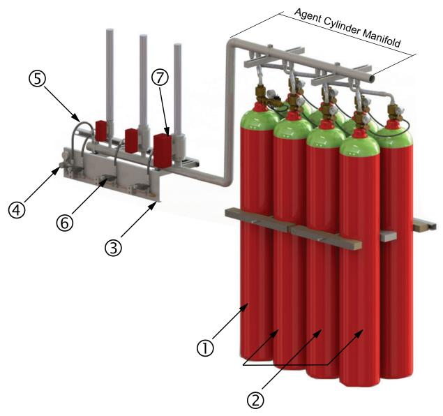
Figure 2. Multi-Hazard System Example
