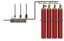
Figure 13. Selector Valve Setup
