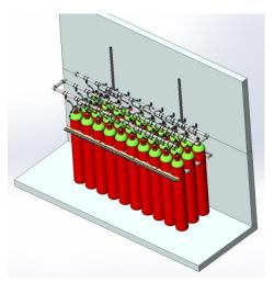
Figure 16. 80L Cylinder Racking Example
